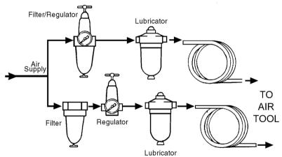
A typical air line layout is shown above. The use of an automatic in-line filter and regulator will keep air tools in good condition. Air compressors must comply with the appropriate European Community Safety Directives. Only clean, dry, regulated compressed air should be used.
